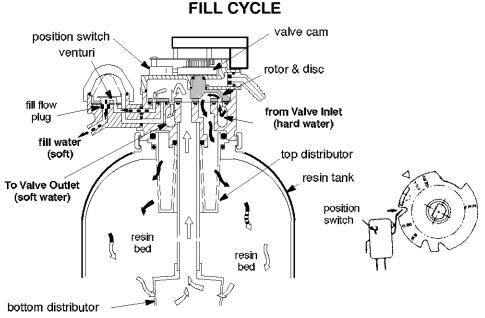
To begin a regeneration, the electronic timer energizes the circuit to the valve motor. The valve motor rotates the rotor and disc and the valve cam until the position switch lever drops, to open the motor circuit and position the valve in FILL. As the rotor and disc rotates, the port opens for SOFT water fill through the venturi. Fill flow continues to the brine valve, and into the salt storage tank. Soft water is still available to the house lines. **5** - **6**
